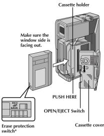
\* **To Protect Valuable Recordings** . . . ....slide the erase protection switch on the back of the tape in the direction of "SAVE". This prevents this tape from being recorded over. If you decide later that you do want to record on this tape, slide the switch back to "REC" before loading the tape.
