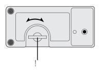
1 JLIP (Joint Level Interface Protocol) Connector Connect to a JLIP-compatible camcorder or VCR to control it from the computer using the provided Software.
