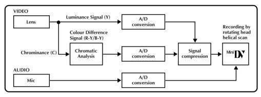
This camcorder separates the data into blocks, writing one block of each data type on each track of the tape.
